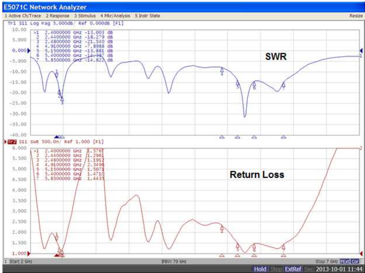
Figure 2 Typical Straight Position Reflection Performance
