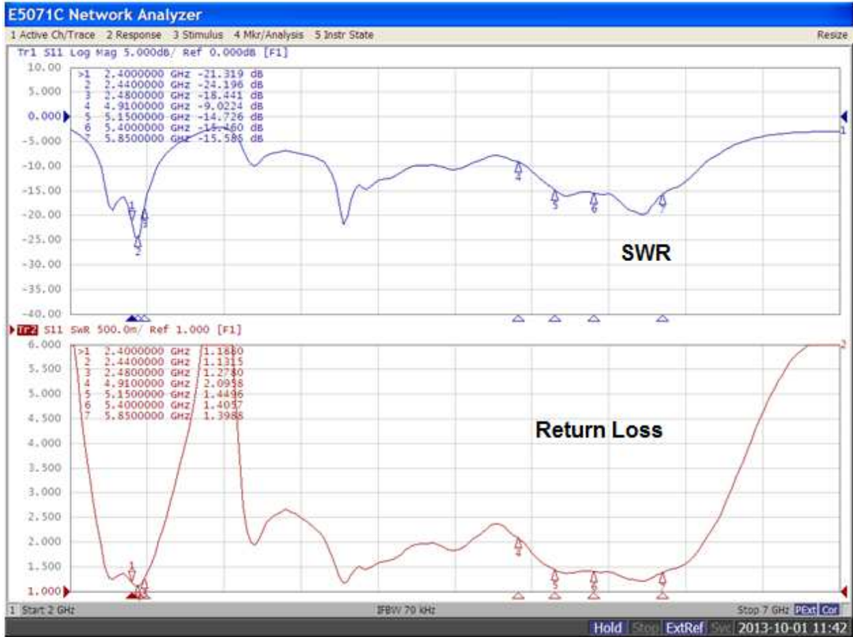
Figure 3 Typical Bent Position Reflection Performance
