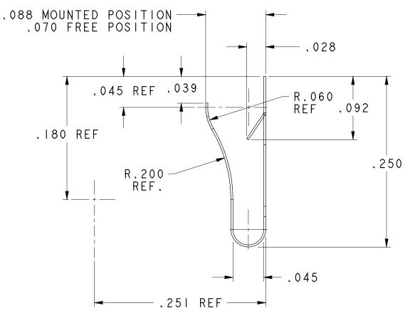
MOUNTED DIMENSIONS ON 18 GAGE SHEET METAL SCALE 10:1
