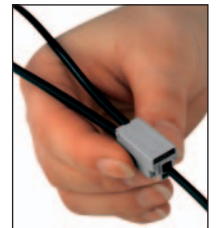
Stranded conductors strip (8–9 mm) conductor, compress terminal and insert conductor
