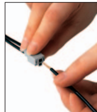
Solid conductor strip (8–9 mm) and connect conductor
