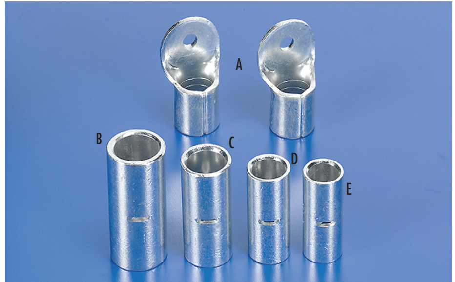
Large Brazed-Seam Terminals: A = 400 MCM Wire Gauge Large Brazed-Seam Splices: B = 500 to 600 MCM Wire Gauge, C = 350 to 450 MCM Wire Gauge D = 300 to 350 MCM Wire Gauge, E = 250 to 300 MCM Wire Gauge
