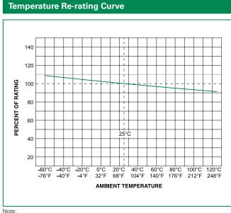
Rerating depicted in this curve is in addition to the standard derating of 25% for continuous operation.
