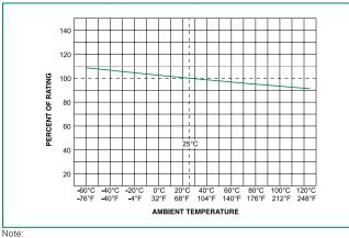
1. Re-rating depicted in this curve is in addition to the standard derating of 25% for continuous operation.
