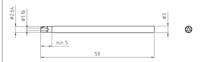
All dimensions are in mm; tolerances according to ISO 2768 m-H
