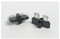
Operating Temp.: -40°C to +125°C Maximum Continuous Load Rating: 35A\* Housing Material: Thermoplastic (UL 94V0 Rated)
