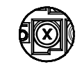
DETAIL 4 SCALE 5:1 INSTALL SEAL PLUG INTO CONNECTOR ASSEMBLY AS SHOWN PER NOTE 4
