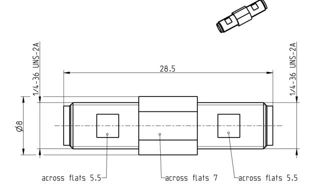
All dimensions are in mm; tolerances according to ISO 2768 m-H
