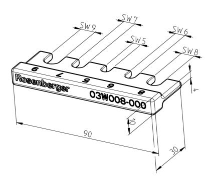
All dimensions are in mm; tolerances according to ISO 2768 m-H
