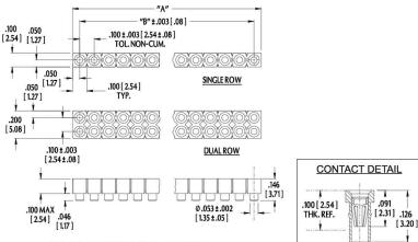
"A"= N0. OF PINS PER ROW x 0.100 [2.54] "B"= (N0. OF PINS PER ROW -1) x 0.100 [2.54]
