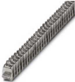
Power terminal block, Connection method Screw connection, Load current : 76 A, Cross section: 1.5 mm 2 - 16 mm 2 , Width: 9.8 mm, Color: silver
