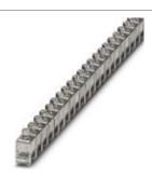
Power terminal block, Connection method Screw connection, Load current : 125 A, Cross section: 2.5 mm² - 35 mm², Width: 14.3 mm, Color: silver
