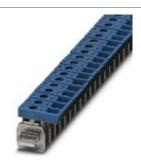
Power terminal block, Connection method Screw connection, Load current : 41 A, Cross section: 0.5 mm² - 6 mm², Width: 7 mm, Color: blue
