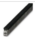
Power terminal block, Connection method Screw connection, Load current : 76 A, Cross section: 1.5 mm² - 16 mm², Width: 9.8 mm, Color: black
