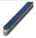
Power terminal block, Connection method Screw connection, Load current : 125 A, Cross section: 2.5 mm<sup>2</sup> - 35 mm<sup>2</sup>, Width: 14.3 mm, Color: blue
