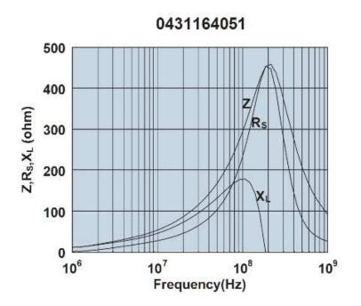
Impedance, reactance, and resistance vs. frequency.
