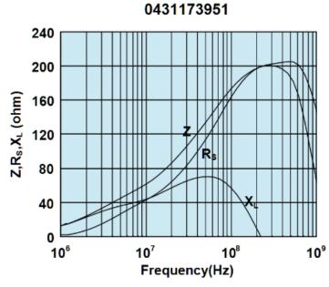
Impedance, reactance, and resistance vs. frequency.
