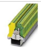
Ground modular terminal block, Connection method: Screw connection, Cross section: 0.2 mm<sup>2</sup> - 4 mm<sup>2</sup>, AWG 24 - 12, Width: 5.2 mm, Color: green-yellow, Mounting type: NS 35/15-2,3
