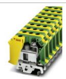
Ground modular terminal block, Screw connection, Cross section: 0.75 mm² - 35 mm², AWG: 18 - 2, Width: 15 mm, Color: green-yellow, Mounting type: NS 35/7.5, NS 35/15, NS 32
