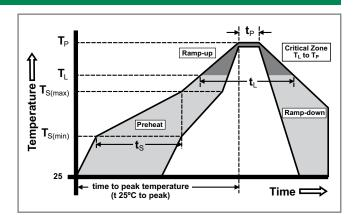
Wave Soldering Parameters
