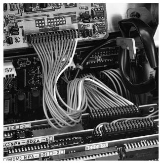
This 2.5mm pitch insulation displacement connector is another version of the NR connector for printed circuit boards. The NRD connector allows daisy chaining and is very useful in simplifying connection systems in electronic equipment.
