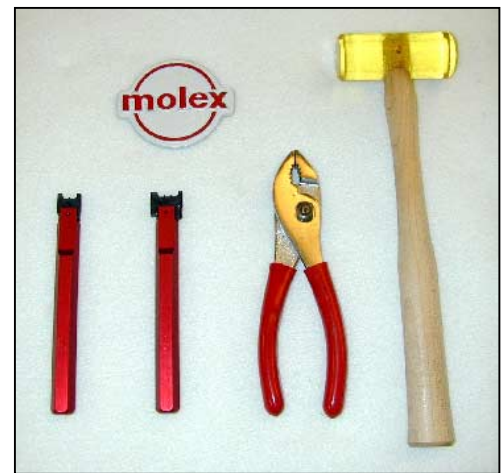
Figure 1-TOOLS NEEDED (From Left To Right: 6-Row Inserter, 8-Row Inserter, Slip Joint Pliers, Plastic Hammer)
