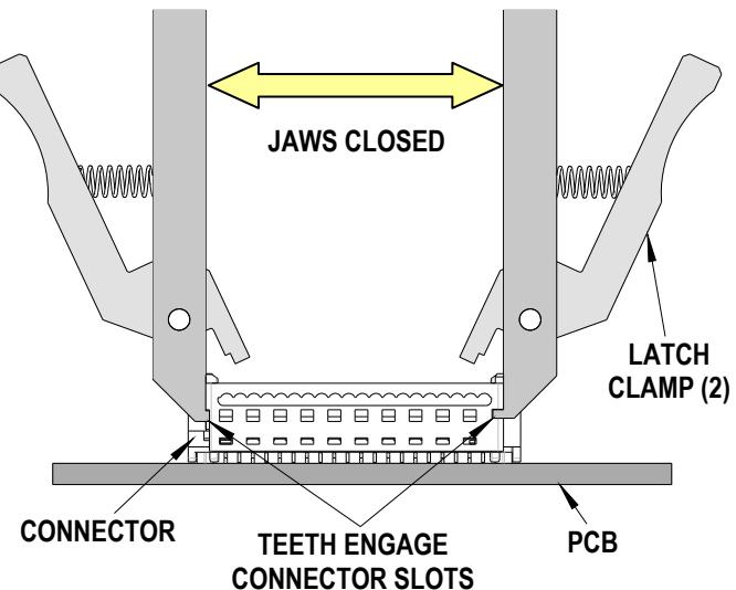
4. While keeping the jaws closed on the connector, squeeze the latch clamps until they stop against the sides of the tool jaws. This releases the header latches so the connector can be removed without latch damage. See Figure 3.
