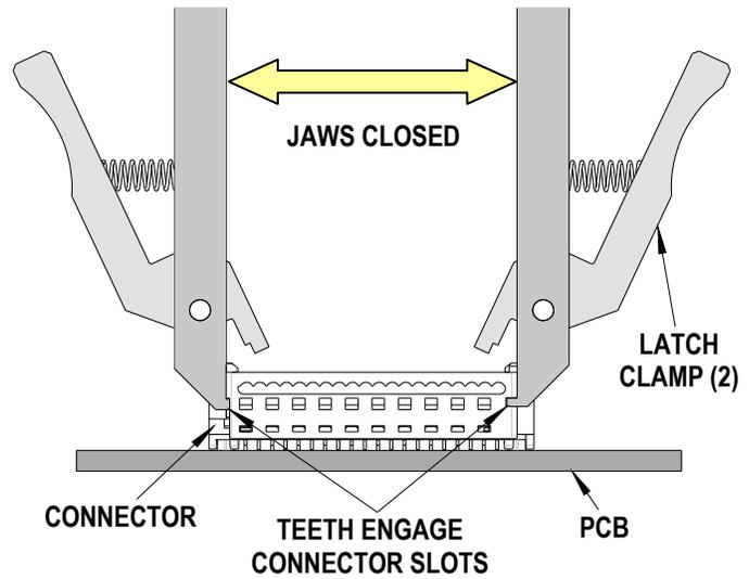
4. While keeping the jaws closed on the connector, squeeze the latch clamps until they stop against the sides of the tool jaws. This releases the header latches so the connector can be removed without latch damage. See Figure 3.
