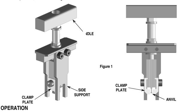
**Note:** Be sure that all parts of the Removal Tool will clear any components on the printed circuit board during use. Tape may also be placed over circuit traces or on the bottom of the side supports for added protection of the printed circuit board.
