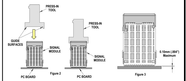
3. Using the application tool and an appropriate press, seat the vertical signal module until there is less than 0.10mm (.004 in) clearance between the bottom of the plastic housing and the surface of the PCB. See Figure 3.
