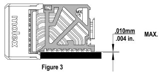
There should be no broken stand-offs along the perimeter of the part (an indication of over-pressing).
