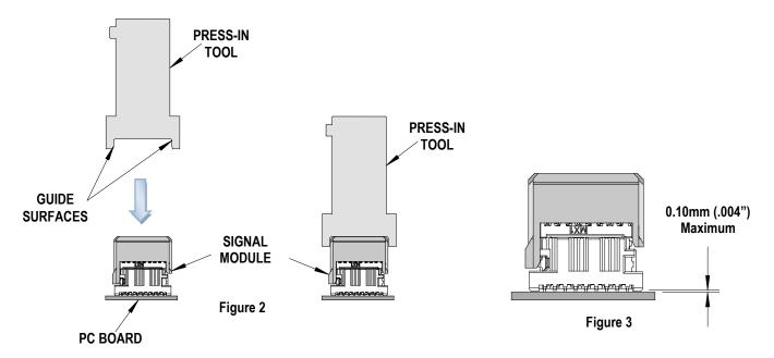
3. Using the application tool and an appropriate press, seat the Signal module until there is less than 0.10mm (.004 in.) clearance between the bottom of the plastic housing and the surface of the PCB. See Figure 3.
