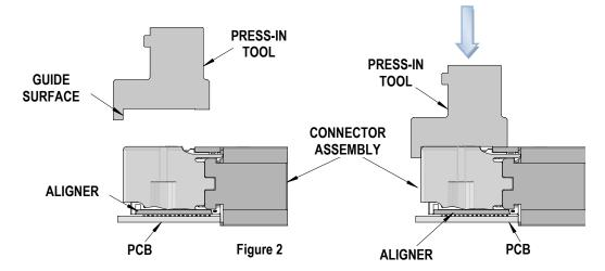
3. Using the application tool and an appropriate press, seat the Orthogonal Direct Ram module until there is less than 0.10mm (.004 in) clearance between the bottom of the plastic housing/aligner and the surface of the PCB. See Figure 3.
