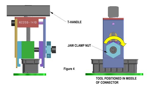
5. To firmly grip the connector, be sure to use the provided wrench to securely tighten the Jaw Clamp Nut. See Figure 5.
