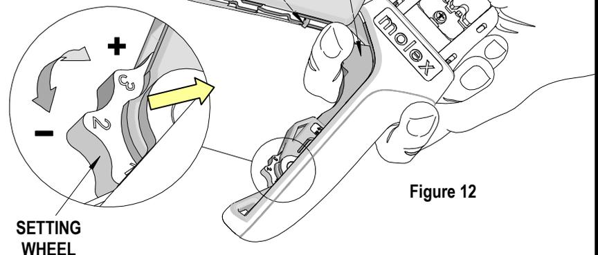
1. Hold the hand tool in the palm of your hand as shown in Figure 10. Using the index finger squeeze the link towards the top of the hand tool frame. This will release the preload adjustment wheel.
