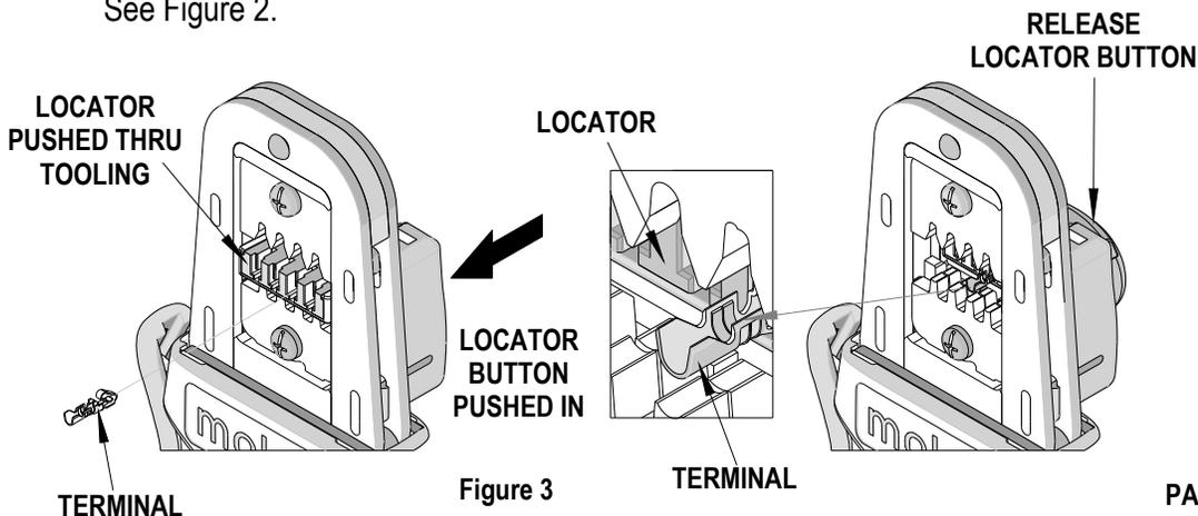
3. While holding the locator button in, load the terminal into the proper nest opening in the locator based on the wire gauge or terminal type markings on the hand tooling. See Figure 3.
