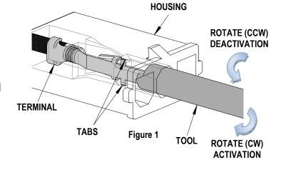
6. Use the 63813-0800 Extraction Tool to extract the terminal from the housing.
