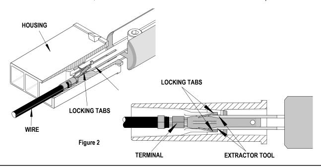
**CAUTION**: This extractor tool should be used to extract the terminal only. Using it for unintended purposes may cause injury or damage to parts.
