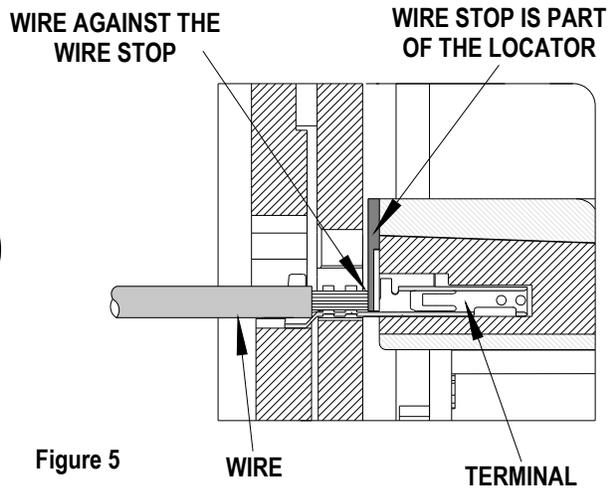
**Note:** The tamper proof ratchet action will not release the tool until it has been fully closed.
