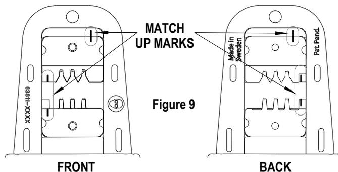
1. The locator must be removed before reversing the tooling.
