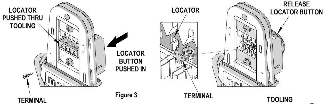
3. While holding in the locator button, load the terminal into the proper nest opening in the locator, based on the wire gauge or terminal type markings on the hand tooling. See Figure 3.
