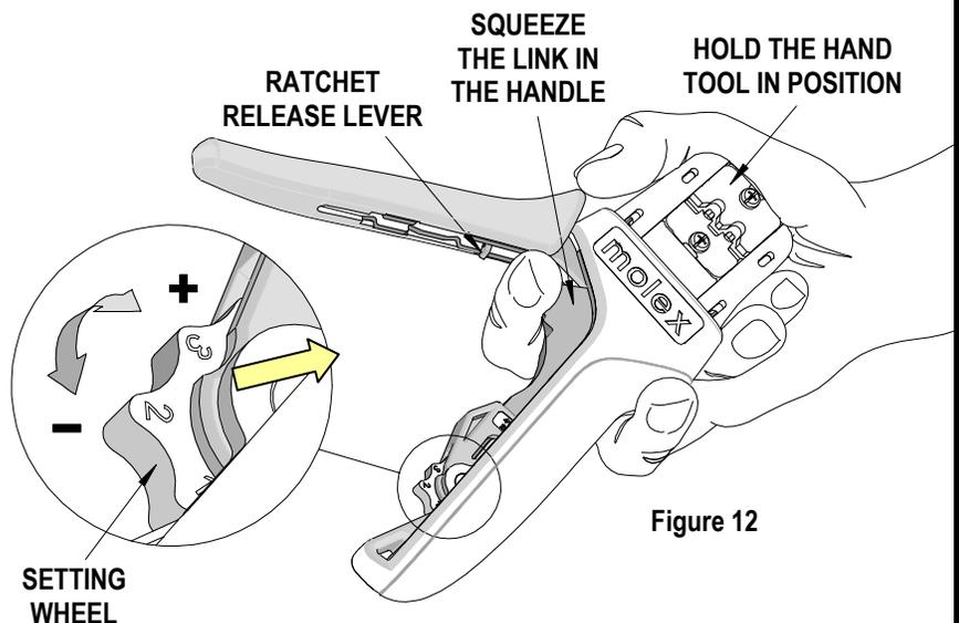
4. Wipe excess oil from hand tool, particularly from crimping area. Oil transferred from the crimping area onto certain terminations may affect the electrical characteristics of an application.
