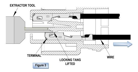
**CAUTION**: This extractor tool should be used to extract the terminal only. Using it for unintended purposes may cause injury or damage to parts. Be careful not to deform the end of the terminal.
