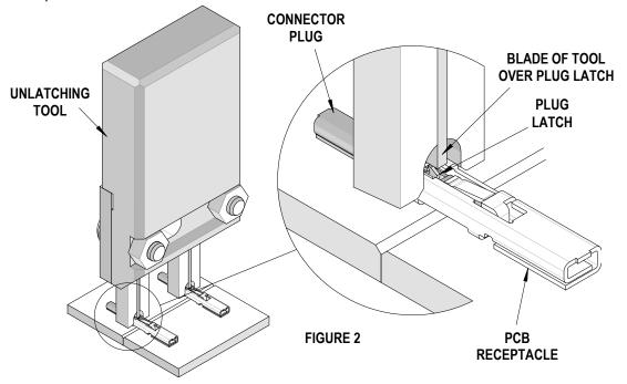
3. Position the tool so that the locating wall (on the inside of the tool), is against the front of the PCB receptacles. See Figure 3.
