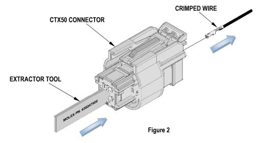
**CAUTION:** This extractor tool should be used to extract the terminal only. Using it for unintended purposes may cause injury or damage to parts. Be careful not to deform the end of the terminal.
