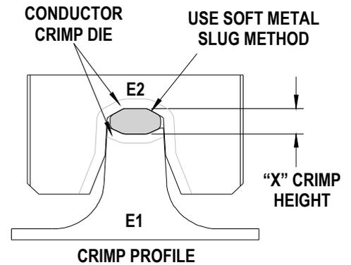
Use soft metal slug (solder) method to measure the "X" dimension. Verify tooling crimp height calibration by referring to the Go/No Go dimensions shown in the chart below.
