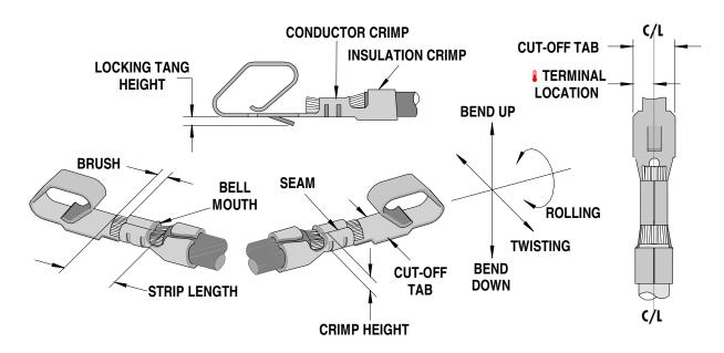
Terminal is to be centrally located between the two (2) cut-off tab edges by one half of the total cut-off tab tolerance.
