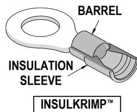
4. The **Avikrimp™** has a color-coded sleeve, which provides insulation as well as an insulation grip. The insulation is made of Nylon, and has a secondary tin-plated brass sleeve added. This brass support sleeve is crimped around the wire
