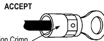
Wire sizes 18 thru 10 AWG require an insulation crimp to securely hold the wire insulation crimp.
