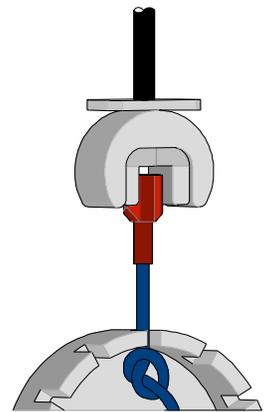
If results of a pull force tests are within an allowed range, it assures that proper crimp force has been applied during crimping. It is crucial as, when making a crimp, enough force must be applied to break down the layer of non-conductive oxides that may build up on the stripped conductor and the tin-plating on the inside of the terminal grip. This is necessary to provide a good metal-to-metal contact.
