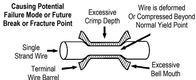
Another way to cause tensile failure is not compressing the barrel enough to hold the conductor securely. Molex crimp tools are designed to eliminate these problems.
