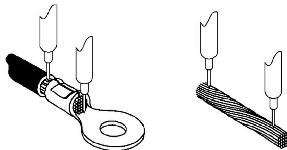
Relative resistance values of less than 1.0 denote a crimped joint with less resistance than the wire; values more than 1.0 indicate greater resistance than the wire. Usually it is easier to measure the voltage drop across the crimped joint. Many specifications state the requirements in terms of voltage drop at a specified current. Voltage drop is the more commonly used term in the industry. If the resistance value is desired, it may be calculated from Ohm's Law:
