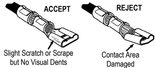
1. Be sure that the contact area is not dented or crushed.
