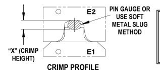
Use gauge pins or soft metal slug (solder) method to measure the "X" dimension. Verify the tooling crimp height calibration by referring to the Go/No Go dimensions shown in the chart below.
