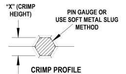
Use gauge pins or soft metal slug (solder) method to measure the "X" dimension. Verify the tooling crimp height calibration by referring to the Go/No Go dimensions shown in the chart below.
