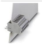
Feed-through terminal block, Connection method: Screw connection, Solder/Slip-on connection, Cross section: 0.2 mm² - 4 mm², AWG 24 - 12, Width: 6.1 mm, Color: gray
