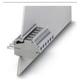
Feed-through terminal block, Connection method: Screw connection, Solder/Slip-on connection, Load current: 18 A, Cross section: 0.2 mm² - 6 mm², AWG 24 - 12, Connection direction of the conductor to plug-in direction: 0  $^{\circ}$ , Width: 6.2 mm, Color: gray
