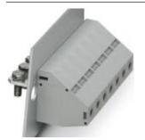
Panel feed-through terminal block, Connection method: Screw connection, Screw connection, Load current: 150 A, Cross section: 16 mm² - 50 mm², AWG 6 - 1/0, Width: 18.8 mm, Color: gray
