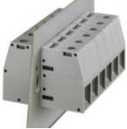
Panel feed-through terminal block, Connection method: Screw connection, Load current : 150 A, Cross section: 16 mm<sup>2</sup> - 50 mm<sup>2</sup>, AWG 6 - 1/0, Width: 18.8 mm, Color: green-yellow
