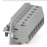
Feed-through terminal block, Connection method: Screw connection, Bolt connection, Load current: 150 A, Cross section: 16 mm² - 50 mm², AWG 6 - 1/0, Connection direction of the conductor to plug-in direction: 0 °, Width: 18.8 mm, Color: gray
