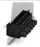
Fuse feed-through terminal block, Connection method: Screw connection, Solder/Slip-on connection, Load current : 6 A, Cross section:  $0.2 \text{ mm}^2$  -  $6 \text{ mm}^2$ , AWG 24 - 12, Connection direction of the conductor to plug-in direction:  $0\,^\circ$ , Width: 12.2 mm, Color: black
